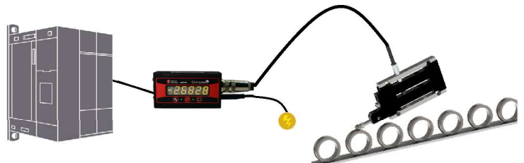
Output to PLC via DC or Modbus
